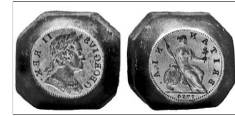
Fig. 2. - Dies for the 1794 halfpenny, with lettering and beading, made with the piece punch in figure 1 (on display in the British Museum).
