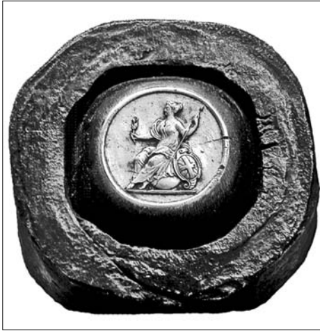
Fig. 1. - Screw press piece punch for the reverse of the 1754 half-penny (on display in the British Museum).
